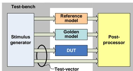
■ A test-bench is a layer of code that is created to apply input patterns (stimulus) to the DUT (design under test) and to determine whether the DUT produces the outputs expected.
