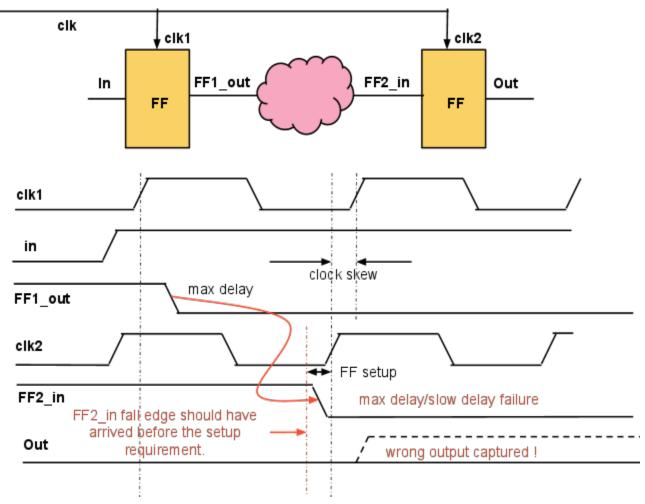
Figure 36. Setup/Max delay failure to a flip-flop.
