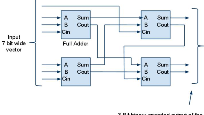
3 Bit binary encoded output of the number of '1's in 7 bit wide input vector
