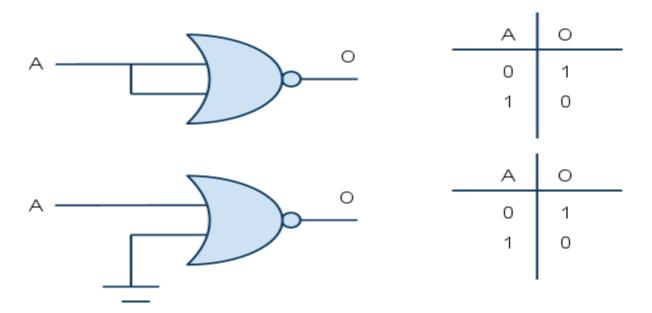
Figure 2. Two input NOR gate as inverter.
