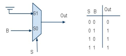
Figure 7. OR using 2:1 MUX
