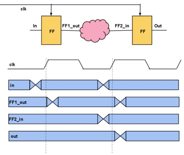
Figure 35. Signal timing propagation from flip-flop to flip-flop
