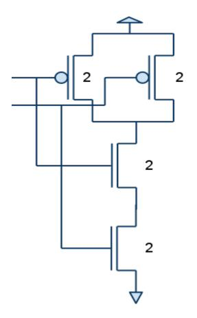
Figure 26. Two input NAND gate.
