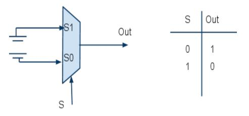
Figure 5. INV using 2:1 MUX
