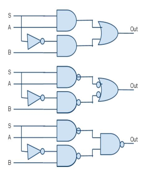
Figure 11. 2:1 MUX using NAND and INV.
