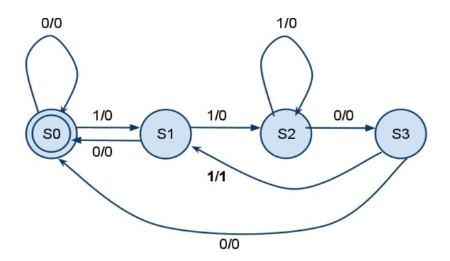
Figure 25. FSM detecting series 1101
