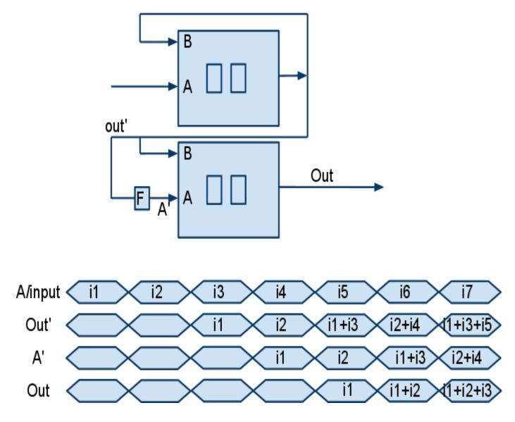
Figure 18. Adder state machine with more clock delay.
