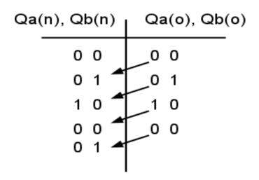
Figure 20. State-transition truth table for 0-2 counter
