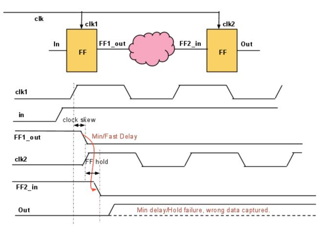
Figure 37. Hold/Min delay requirement for a flop.
