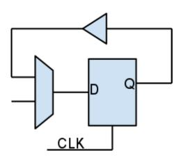
Figure 38. Hold/Min delay requirement for a flop.
