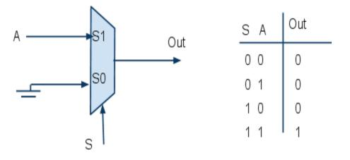
Figure 6. AND using 2:1 MUX
