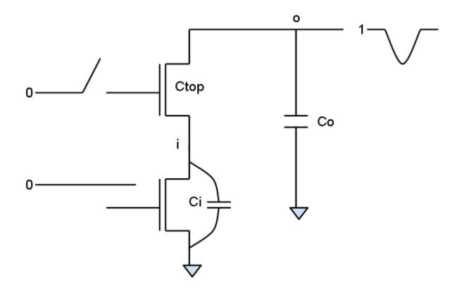
Figure 32. Charge sharing in stacked CMOS gates.
