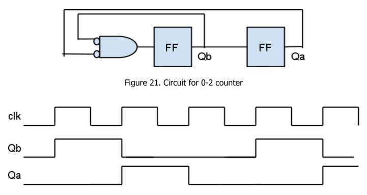
Figure 22. Clock and data waveforms for 0-2 counter
