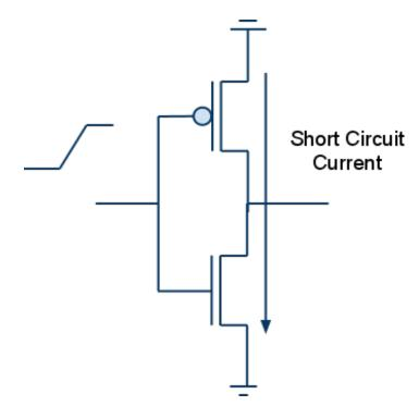
Figure 29. Short-circuit current.
