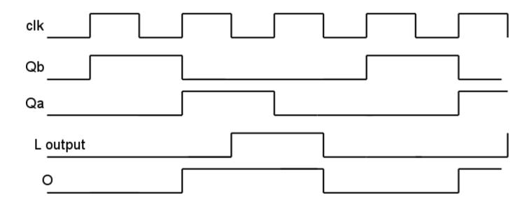
Figure 24. 50% duty cycle divide by '3' clock generator waveforms
