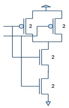
Figure 27. Two input NAND gate with P/N skew of 2/1.
