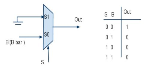
Figure 8. NOR using 2:1 MUX
