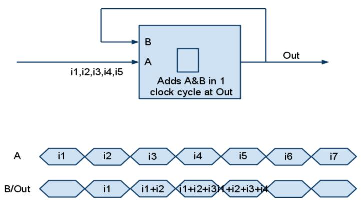
Figure 17. Adder state machine with specified delay.
