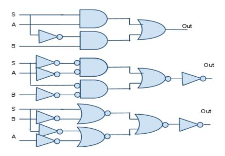
Figure 11. 2:1 MUX using NOR and INV.
